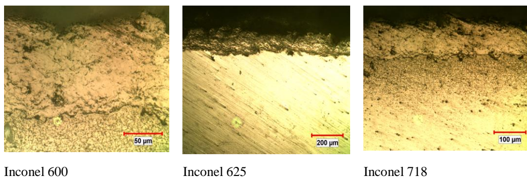
Fig.19 Optical micrographs showing microstructures of coated Inconel 600, 625 and 718
