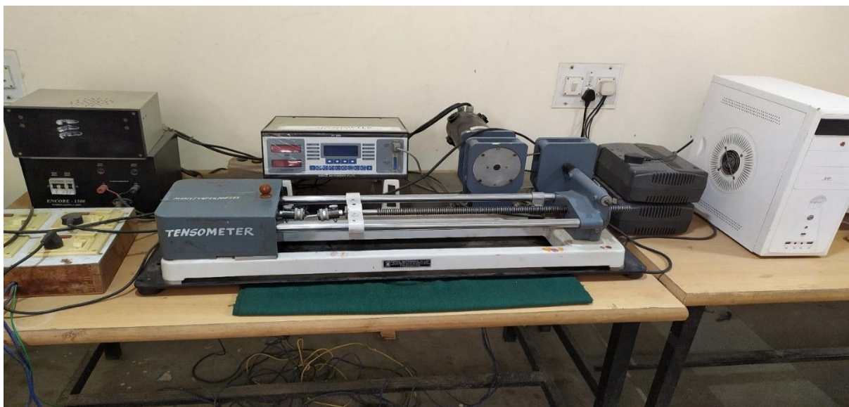
Fig 5: Tensometer setup for finding young's modulus.
