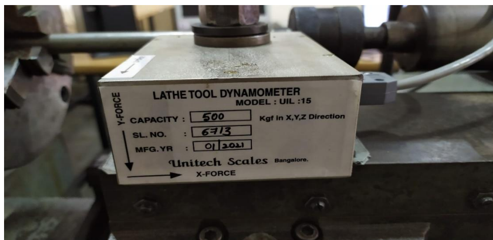
Fig 7: Lathe tool dynamometer setup.
