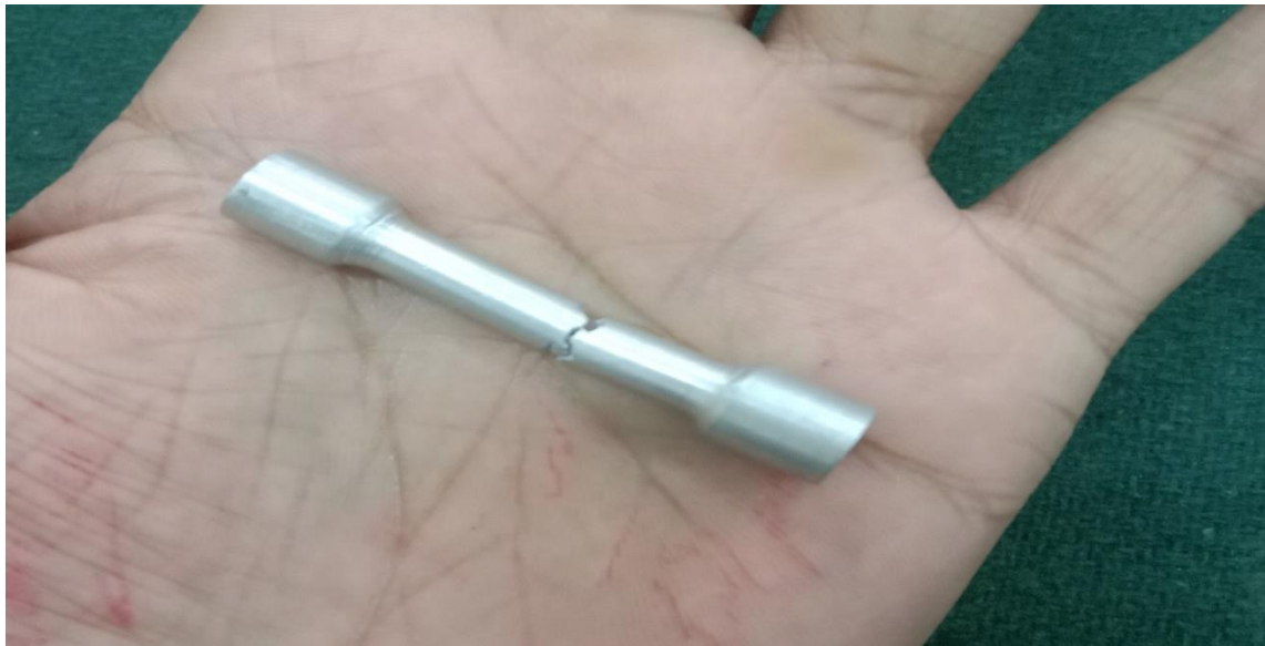
Fig 6: Tensometer specimen prepared in turning operation
