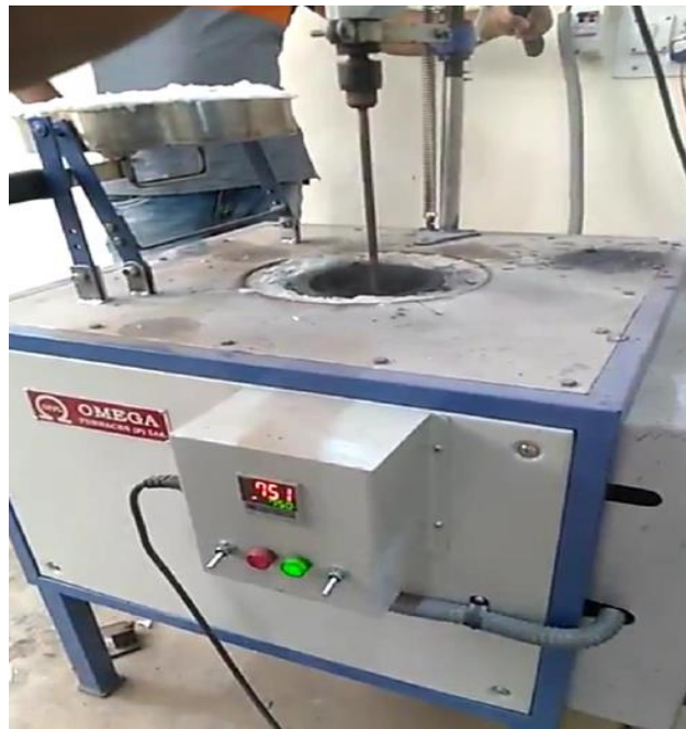
Fig 2: Stirr casting of hybrid composite in a furnce
