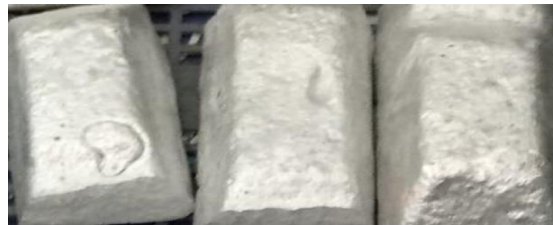
Figure 1: Aluminium 7050 alloy ingot
