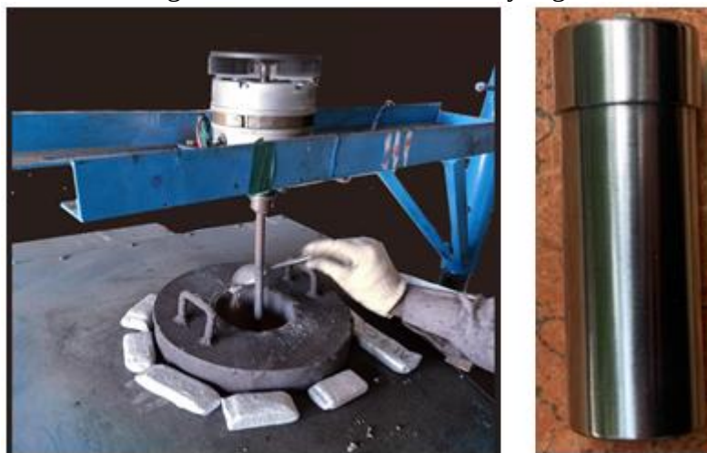
Figure:1(b) Addition of reinforcement during stir casting process (c) Friction Stir Welding (FSW) tool
