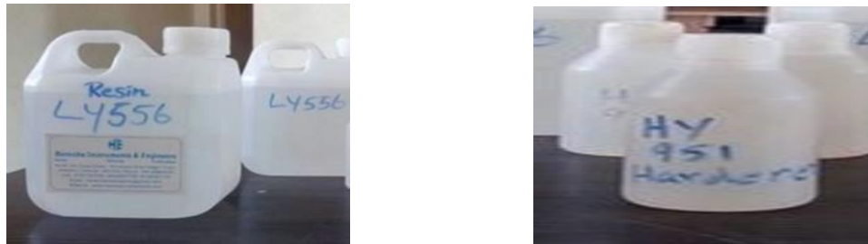
Figure 2: Epoxy resin (LY 556) and hardener (HY 951) used as the matrix material.
