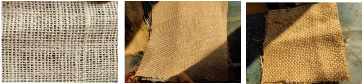
Figure 1: Sisal, kenaf, and camel hair fibers used as reinforcements in this study.
