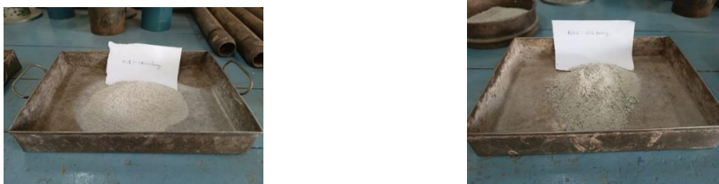
Figure 1. Recycled concrete dust with a maximum size of 1.18 mm (left) and 2.36 mm (right)
