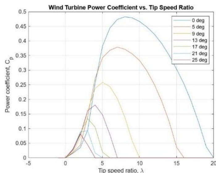
Figure 4: Wind turbine power coefficients C_p as a function of \lambda and \beta .
