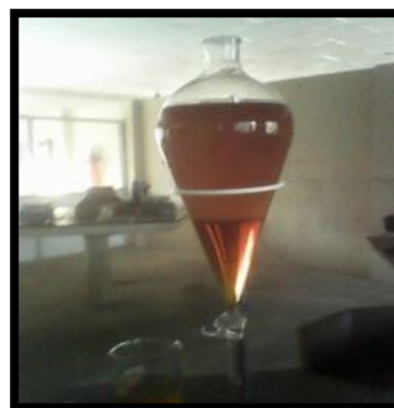
Figure 5. Mixing Methoxide with Rice Bran oil, and decanting to separate glycerin
