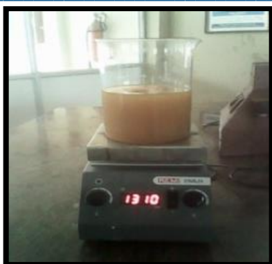
Figure 4. Acid Treatment and Decantation for separation of glycerine
