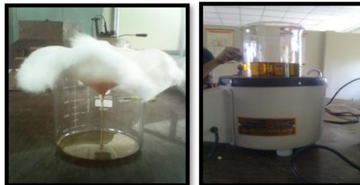
Figure 3. Filtering the oil and Pre-heating it
