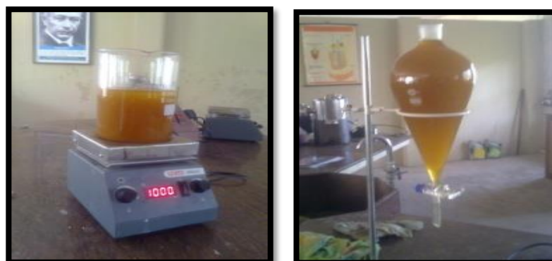
Figure 3. Filtering the oil and Pre-heating it
