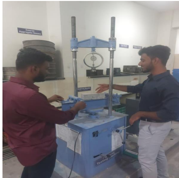
Fig 5.9 – Flexural-strength testing of prism
