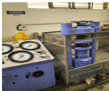
Fig 5.8 – Cylinder testing in Compressive testing machine
