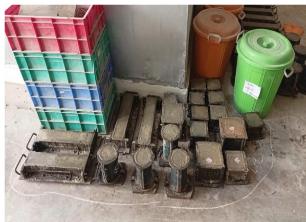
Fig 5.2 – Casting of Normal Cubes, prisms and cylinders
