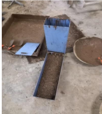
Fig 5.6 L – Box test
