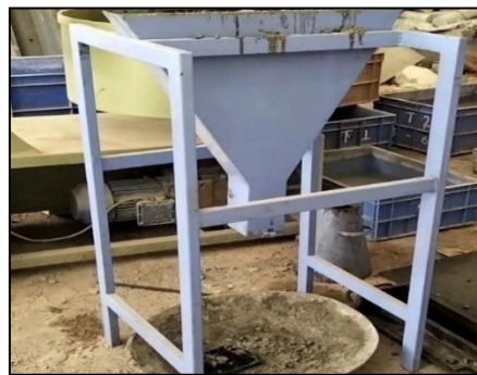
Fig 5.7 V – funnel test
