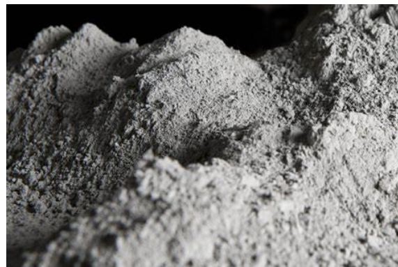
Fig 4.2 - 53 Grade Ordinary Portland Cement
