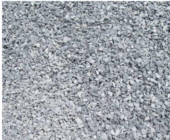
Fig 4.7 – Coarse aggregate (12.5mm down size)
