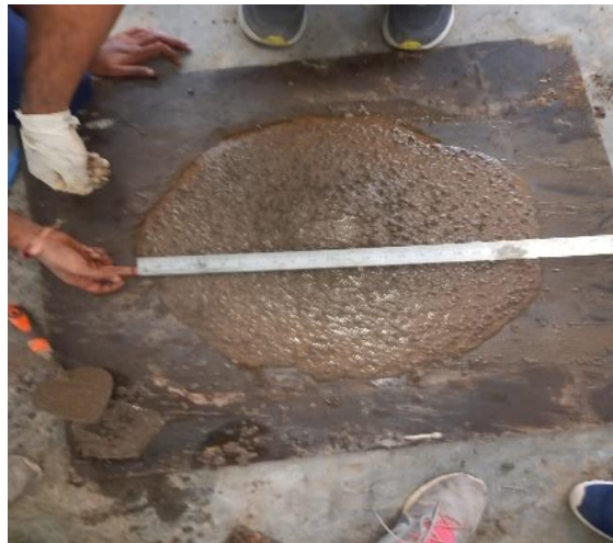
Fig 6.2 – Slump flow of IOT based SCC with 1.5% SP dosage
