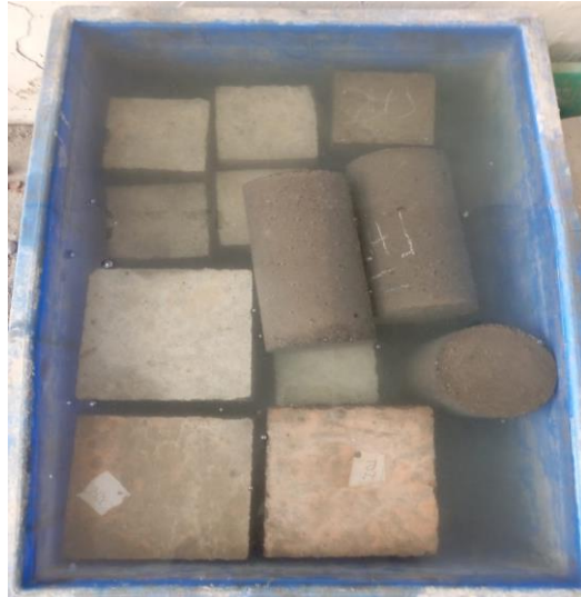
Fig 5.4 – Curing of samples
