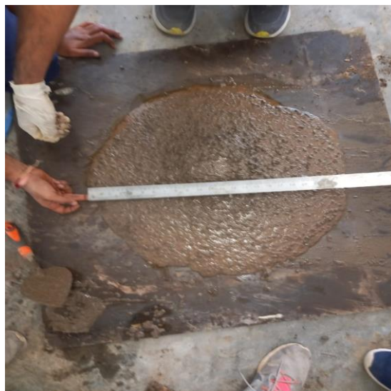
Fig 5.5 – Slump flow test
