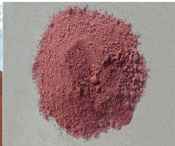
Fig 4.5 – Iron Ore Tailing
