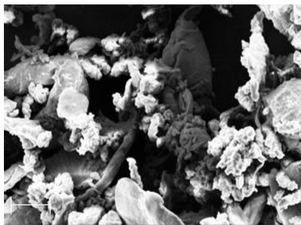
Figure 9. Scanning electron microscope images of TPU/rGO nanocomposite with 1 wt % of reduced Graphene oxide (wet mixing)
