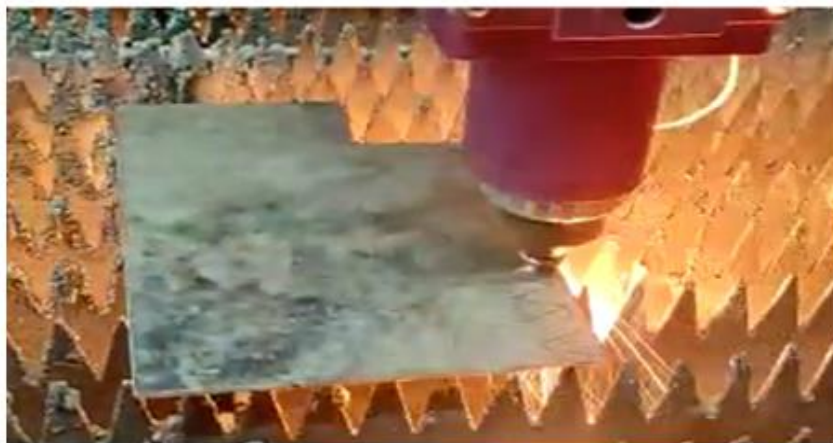
Figure 2: Position of the nozzle of laser beam cutting machine during the cutting operation
