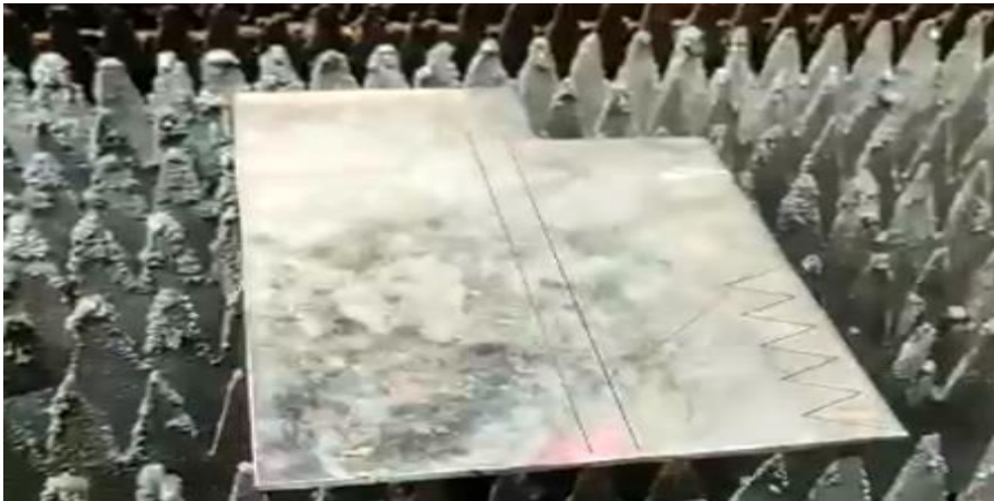
Figure 1: Inconel 718 sheet setup on equipment bed for straight and zigzag cut
