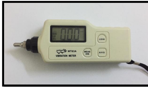
Fig. 6. Wt63a vibration meter was used in the study.
