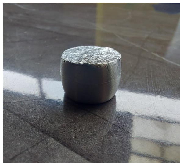
SEM was used to examine the rupture that happened. All Fig. 11: Compressed Steel Specimen
