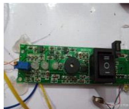
Figure.13 Metal Detector OFF condition
