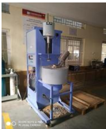
Figure.3. Experimental setup of stir casting process
