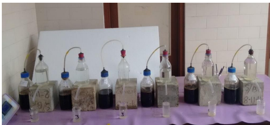
Figure .1 Anaerobic batch reactors setup for various mixing proportions and pH
