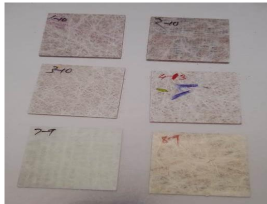
Fig. 1(b) Laminate Natural and Synthetic fiber composite.
