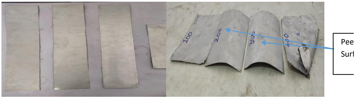
Figure.4 Al5083 As received and shot peened sheets
