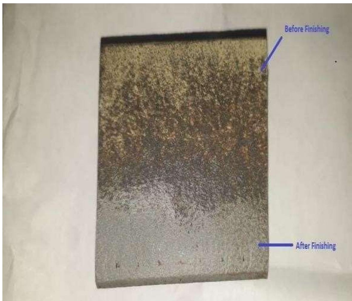
Figure-5. Sample Before and After Finishing At 7 Bar Pressure
