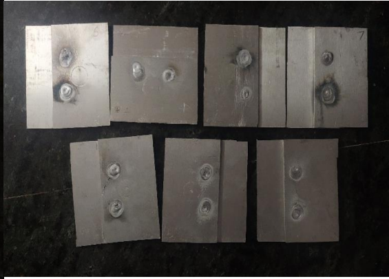
Figure 4: Welded Plates of different parametric inputs
