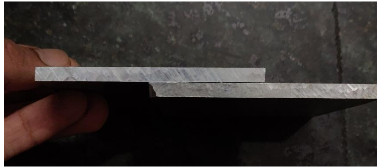
Figure 5: Plug weld- Side View
