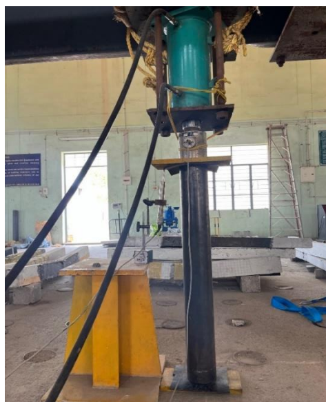
Fig 7 Test setup for CFST column under axial loading
