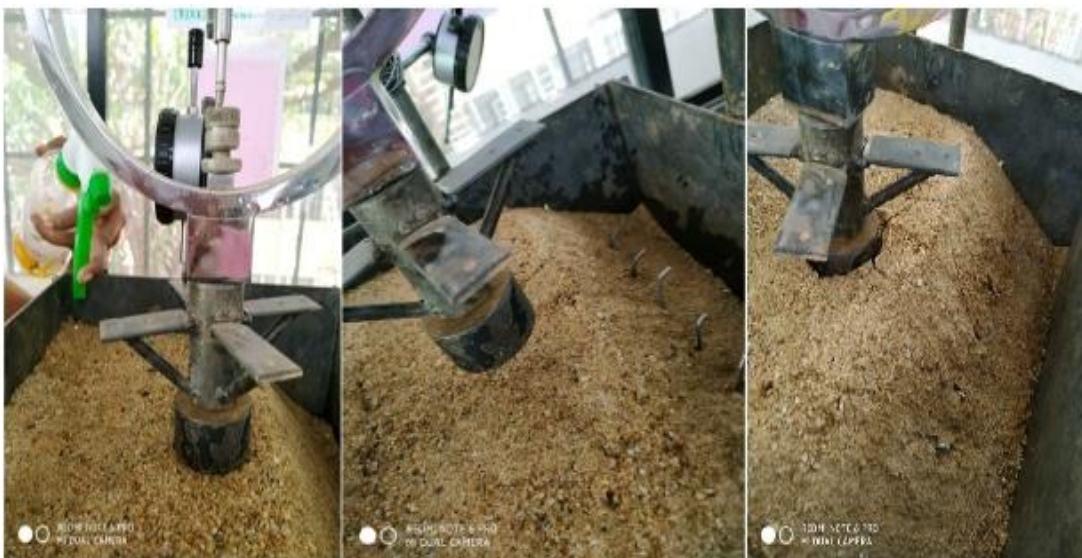
Figure 3 Effect of loading on the 5\text{ mm} away from edge of footing with optimum reinforcement (before and after failure in a saturated sand bed)
