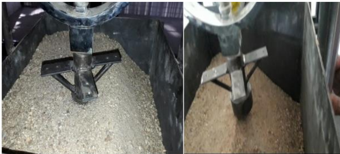
Figure 2 Effect of loading on surface footing resting on sloping ground before and after failure
