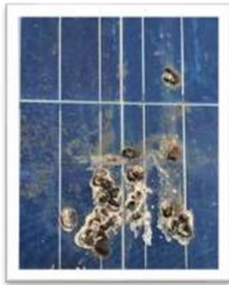
Fig.04 Solar Panel with Dirt
