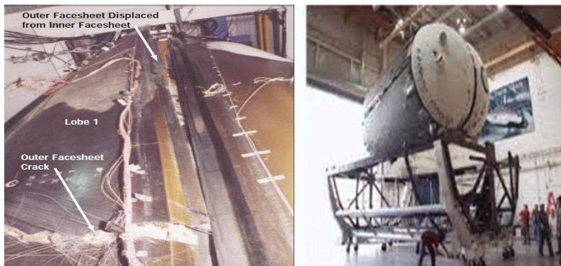
Figure 2: shows the damaged X-33 cryogenic tank [57].
