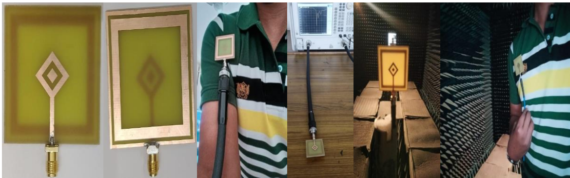
Fig. 2. Proposed microstrip antenna sensor Fabricated and Measured Views
