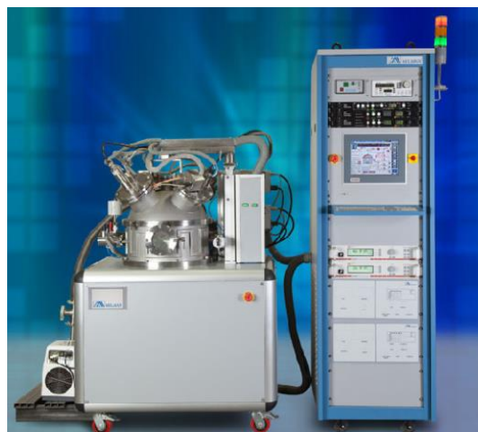
Figure 2: Sputtering machine used in making circular waveguide.
