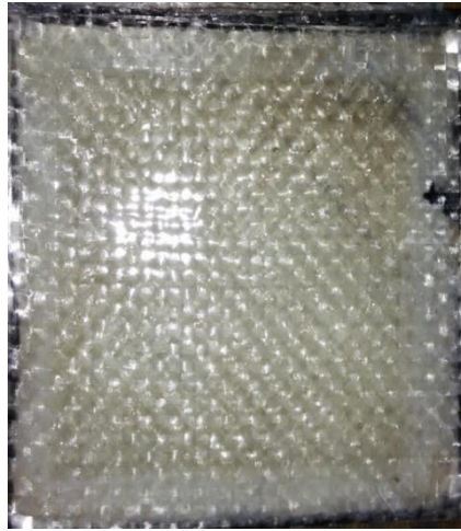
Figure 3: Smart laminate composite after curing.
