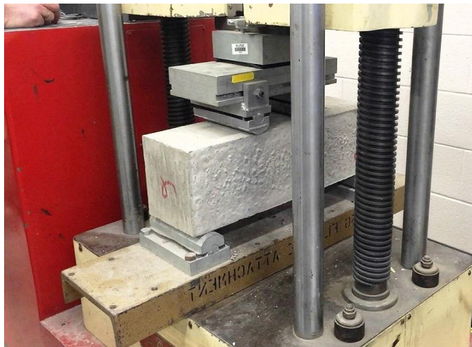
Figure 3: Flexural Strength Test Apparatus
