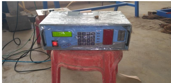
Figure 5: Exhaust flue gas analyzer
