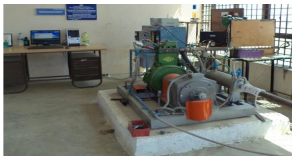
Figure 3: The computerized diesel engine test setup with data acquisition system
