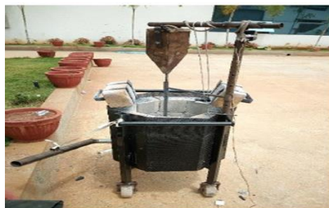
Figure 1: Stir casting setup
