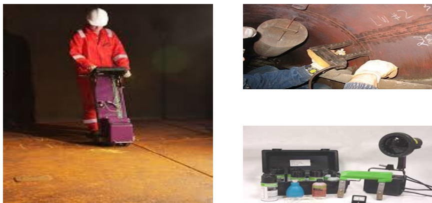
Figure 2. Magnetic flux leakage and yoke
