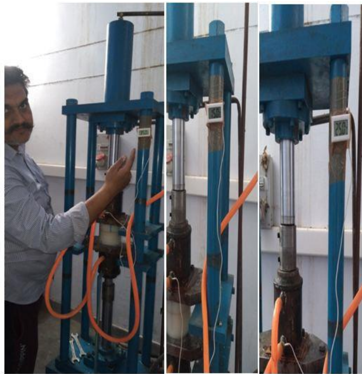
Fig. 2. Developed Thermal-AFM setup at (Yadavindra Department of Engineering, Talwandi Sabo). The media temperature is maintained at 15°C, 25°C & 35°C.
