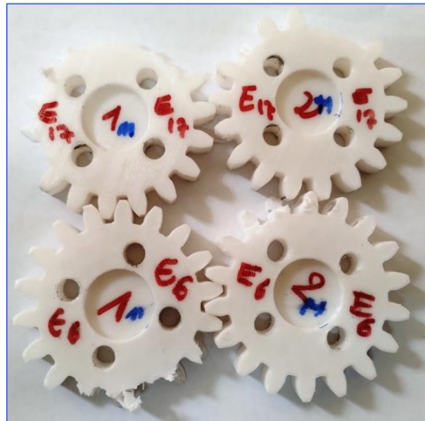
Fig. 4: The sample of test no. 6 and no. 17 (1: The drive gear and 2: The driven gear).
