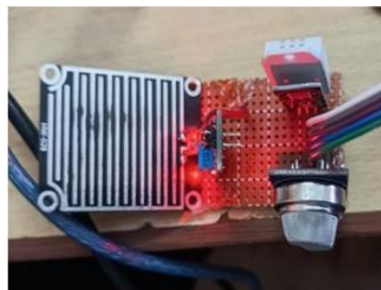
Figure 7 Outdoor module with MQ135, DHT22 and rain sensor
