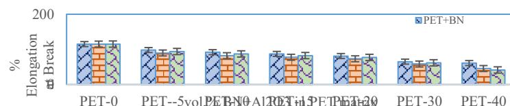
Fig. 3.6, Percent elongation at break of PET+BN, PET+ \text{Al}_2\text{O}_3 and PET-BN+ \text{Al}_2\text{O}_3 Composite
