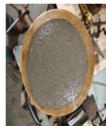
Spread of mortar after flow test
