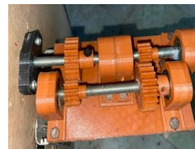
Fig. 1(g): Step-up gear train
