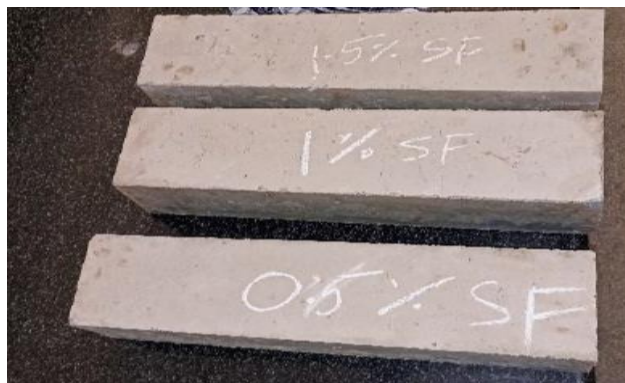
Figure 3. Flexural Strength Test Specimen
