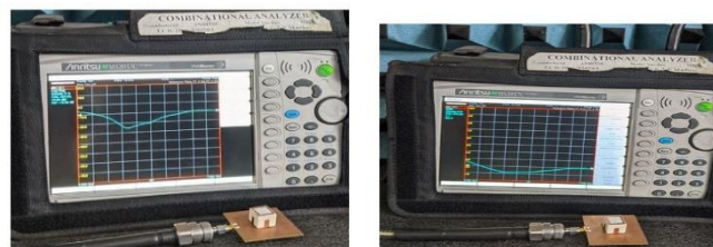
Fig.5. STSSRR with RDRA (a) Measurement setup for Reflection coefficient (b) Measurement setup for VSWR
