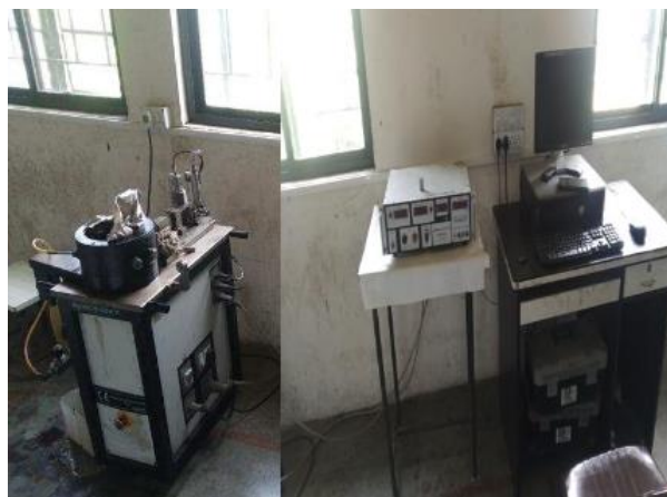
Figure 3. Tribometer experimental test setup
