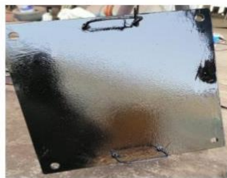
Fig. 3 Photographic views of the steel moulds to prepare sample laminates.
