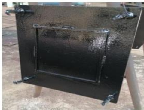
Fig. 3 Photographic views of the steel moulds to prepare sample laminates.
