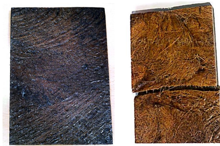
Fig. 10 Flexural failure of the tested samples
