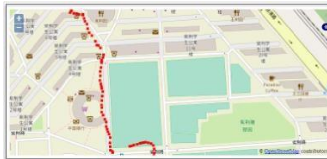
Fig 9. Trip converted to sequence of network edges using map matching
