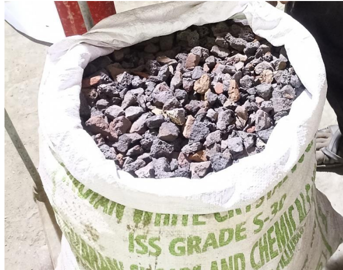
Fig.1 Crushed Over Burnt Clay Bricks
