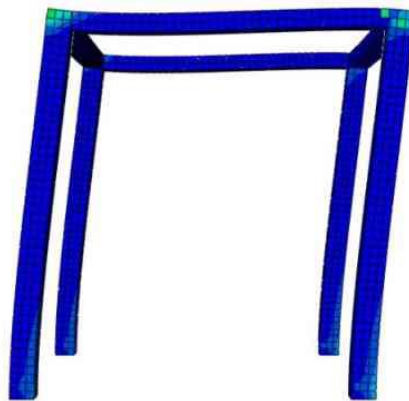
Figure 15: The position of the plastic hinge in the reinforced HPFRCC frame (RH).
