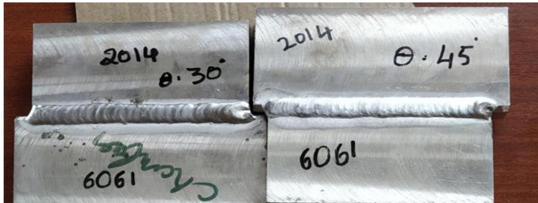
Fig 3: weldments for 30- and 45-degree angles
