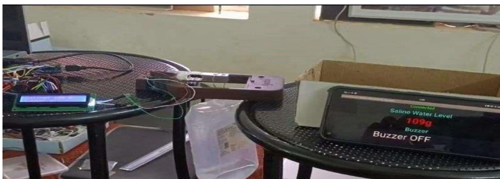
Figure 4 Working model of blood reversal prevention in IV therapy when buzzer is OFF
