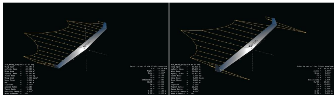
Figure 11. Induced Drag profile on Wing with Winglet at 60 and 90 degrees respectively
