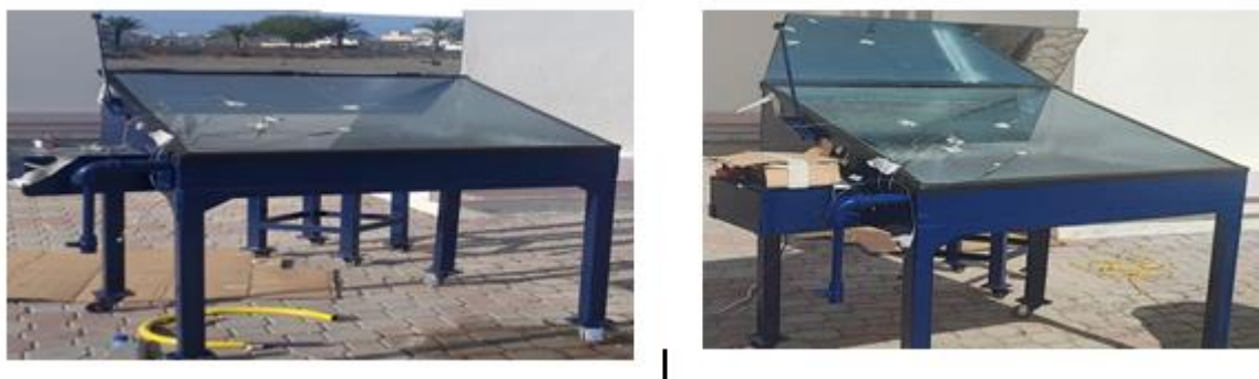
Figure 1: Typical pictures of fabricated solar still
