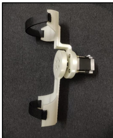
Figure 4: 3D printed exoskeleton structure with stepper motor
