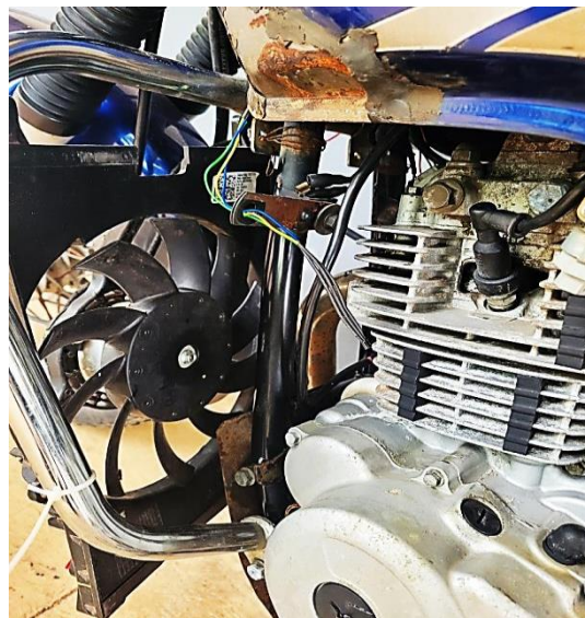
Fig 4: Experimental setup with radiator fan angled towards cylinder fins
