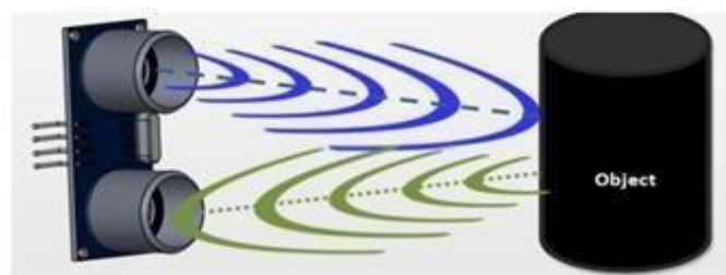
Fig2.Ultrasonic distance device transmitting and receiving ultra sound wave patterns
